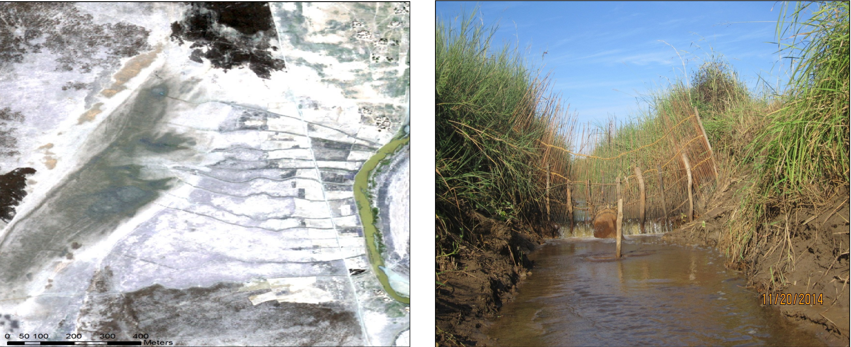
Fig. 1 Canals link depressions to river (L) and channel water and fish through them (R).
